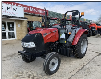
New Case IH Farnall 55A, 2wd, 8x8 gearbox with mechanical shuttle, 2 mech spools, 540 PTO, ROPS. POA
